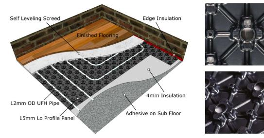
The **TechnoLo** Low Profile Underfloor Heating Panel is 15mm deep, 1050mm long and 650mm wide, giving an area of 0.6m<sup>2</sup> coverage per sheet. It is supplied with a self-adhesive backing ready to be secured to the 4mm insulation.
