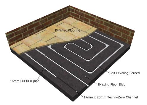
The **TechnoZero** Zero Depth Retrofit Underfloor Heating pipework is fitted into channels cut into the existing screed floor without adding any depth to the existing floor construction. **TechnoZero** channels can even be cut through existing tile or stone flooring.
